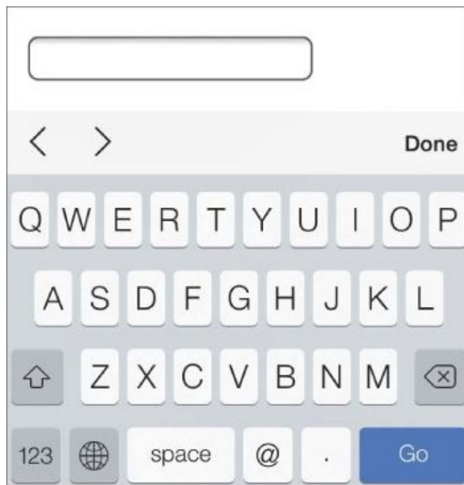
Figure 10.4 iOS7 controls for an <input> element with a type attribute value of email
