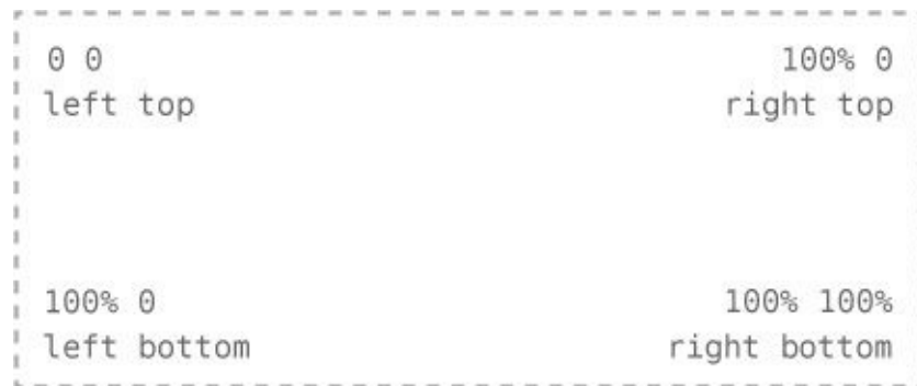
Figure 7.1 Background images are positioned from the left top corner of an element
