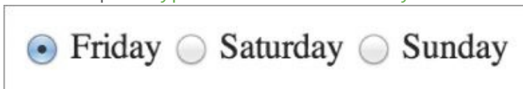
Figure 10.9 A group of radio buttons created by way of the <input> element with a type attribute value of radio
