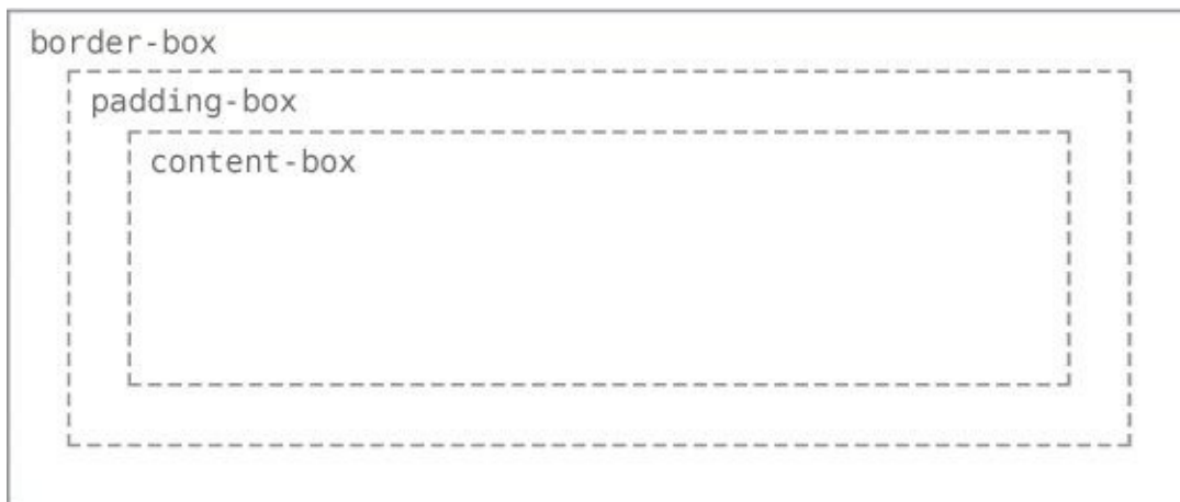
Figure 4.6 Different box-sizing values allow the width of an element—and its box—to be calculated from different areas
