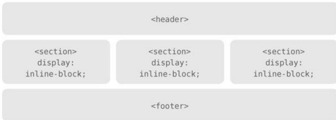
Figure 5.9 A three-column page layout using inline-block elements with properly removed white space
