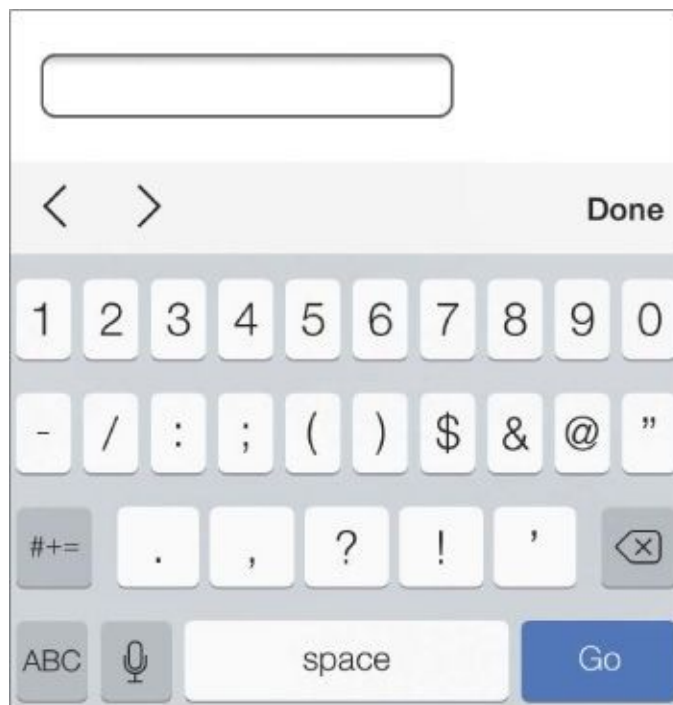
Figure 10.6 iOS7 controls for an <input> element with a type attribute value of number
