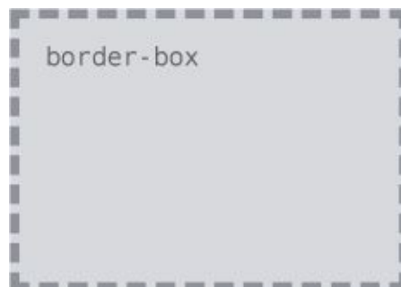
Figure 7.13 The border-box value extends the background into the border of an element
